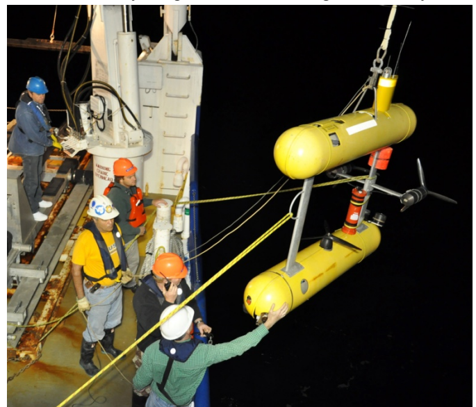
Figure 1. Mola Mola AUV during deployment operations
