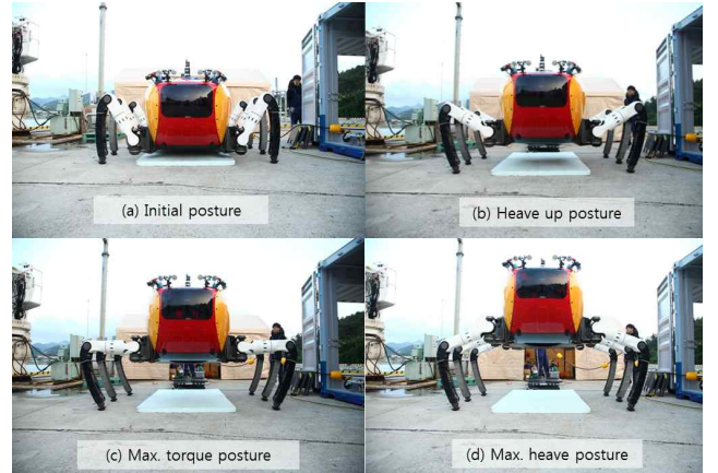
Fig. 7 Extreme motion with full loads to verify the capacity of legs.
