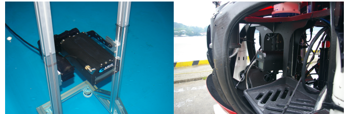
Figure 1 (Left) ARIS with X2 rotator for roll/tilt mode (Right) ARIS and X2 rotator installed on CR200
