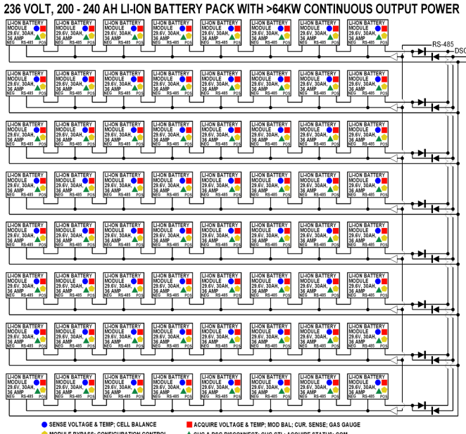
Figure 3. Example Distributed Architecture Lithium-Ion Battery System
