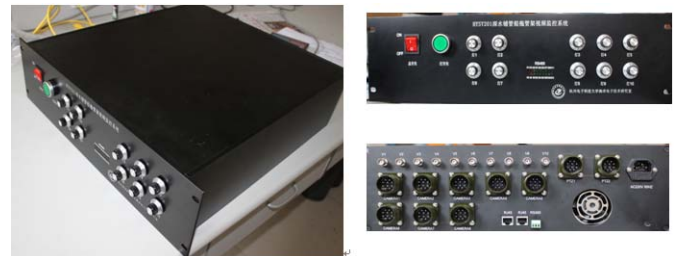
Fig. 6 The deck junction box
