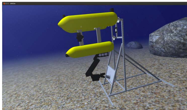
Fig. 1. UWSim visualization of the underwater considered scenario with the I-AUV docked in the intervention panel designed by UdG.
