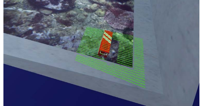
Fig. 6. Structured light through laser calculation in UWSim, for recognizing a black box in the sea bed
