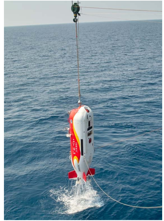
Fig. 6. Recovery of the AUV "JINBEI" hung and hoisted at one-point.
