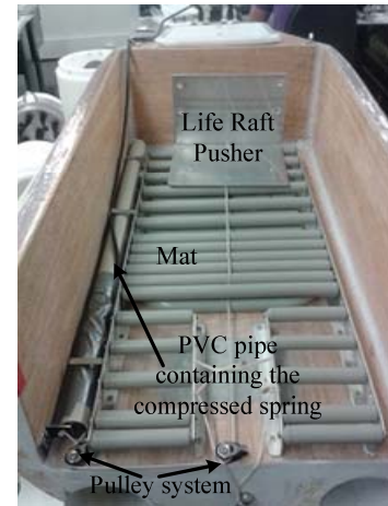
Fig. 4 - Life Raft deployment system.
