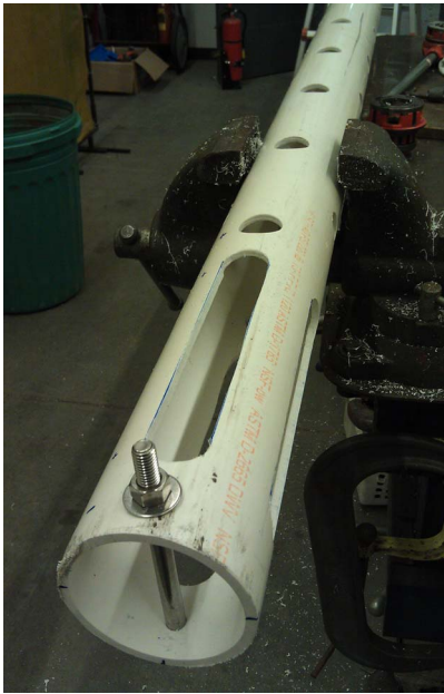
Fig. 2. One of the PVC wells that house the test sensors shown here during fabrication. The base of the water quality sonde rests against the bolt and the large holes allow sufficient water to flow past the probes.
