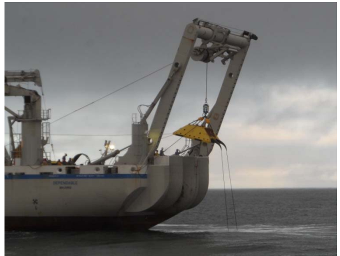
Fig. 11. Node Installation from TE SubCom Cable Ship CS DEPENDABLE
