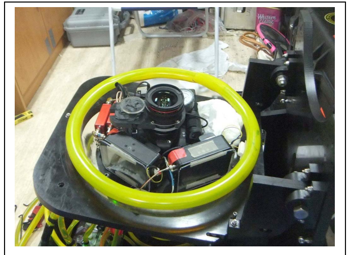
Fig. 3. With the upper polished hemisphere removed, the interior is easily seen. The Canon 5D camera is centered on apex of the dome. The focus gear is to the left. Two Atomos Samurai video recorders, located at the bottom of the image, capture the images from the stereo camera pair located on the baited drop arm. (Photo used with permission, Earthship Productions.)
