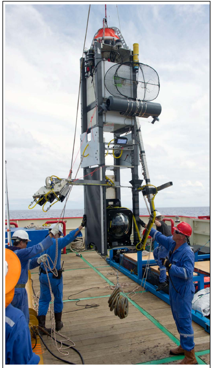
Fig. 1. The Alpha Lander, DOV MIKE, is lifted by crane during deployment. Steel barbell weights are the clump weight. The drop arm, retracted against the face of the lander during deployment, holds a Niskin bottle rigged as an animal trap, and a net fish trap. A stereo camera pair is mounted to the drop arm, and looks upward in this view. The polished glass camera sphere is located at the bottom. Small barbell weights are fixed to the underside of the aluminum deck below the camera housing to negate the buoyancy of the camera sphere for overall vehicle stability. A fixed light arm holds the 3-element key light to the right and forward of the camera. A single-element fill light is positioned mid-body directly over the camera sphere. Fixed and variable buoyancy modules made of syntactic blocks are located above this. The Command/Control sphere tops the stack, with an aluminum lifting bale and hardhat segment providing cover and protection. (Photo used with permission, Earthship Productions.)
