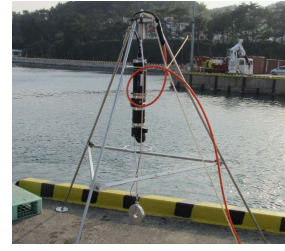
Fig. 4. Tripod with 1171 high resolution scanning sonar
