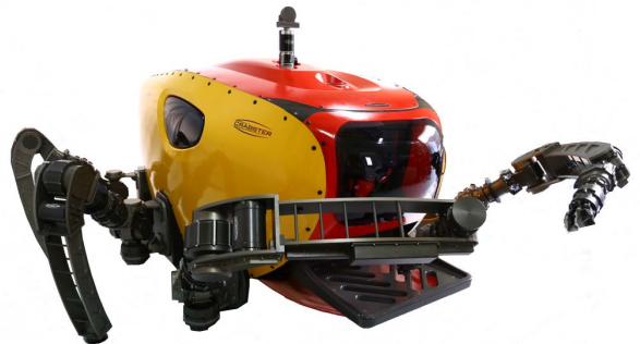
Fig. 1. Appearance of subsea walking robot CR200.
