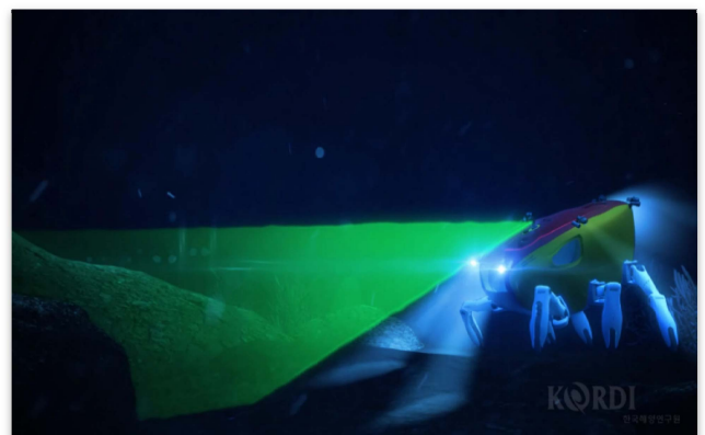
Fig. 2. Scanning concept of CR200
