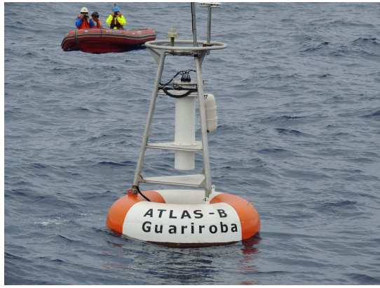
Fig. 2. The Atlas-B buoy Guariroba just after its mooring at 28.5°S, 44°W.
