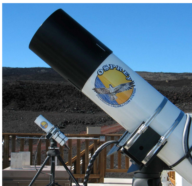
Fig. 7. Synchronous measurements of shrouded (foreground) and unshrouded (background) sky radiance were made at Mauna Loa Observatory (MLO). Radiance instruments are mounted on a military-grade, commercial-off-the-shelf (COTS) tracking system.
