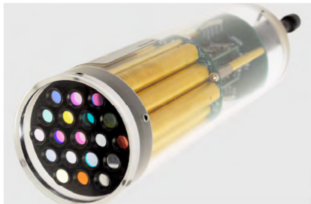
Fig. 2. A 19-channel radiance sensor built from microradiometers (the clear acrylic housing is for demonstration purposes only). The microradiometers are encased in brass cylinders and located between the aperture window (with colored filters visible) and the green aggregator and support electronics boards.
