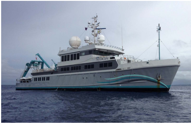
Fig. 5. The M/V Alucia is 183 ft. with a gross tonnage of 1396 tons and outfit as an expeditionary yacht, capable of oceanographic research. In this case, the Nereus system was mobilized onboard. The vessel possesses twin screws and a bow thruster, but is not equipped with dynamic positioning.
