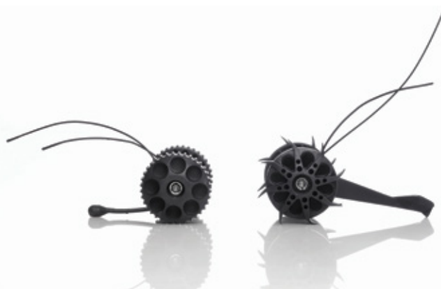
The ruggedized search and rescue version of the Scout features spiked wheels for climbing over obstacles. (PHOTO COURTESY RECONROBOTICS INC.)
