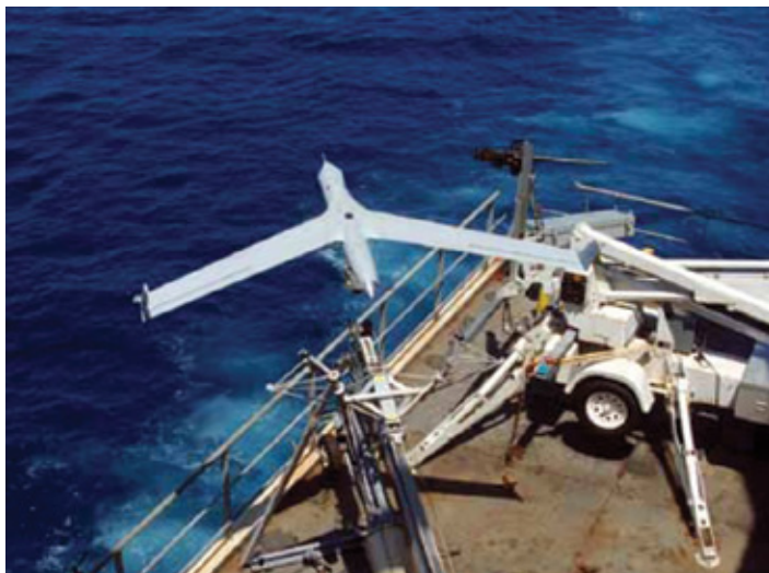
Ultralight UAVs are launched by catapult, suffering 35 Gs of force. (COURTESY OF INSITU INC.)
