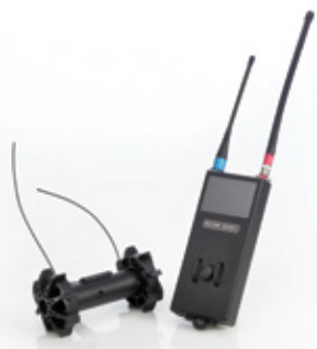
The Recon Scout IR features a visible/IR sensor mounted in the crossbar and a handheld control unit. (PHOTO COURTESY RECONROBOTICS INC.)
