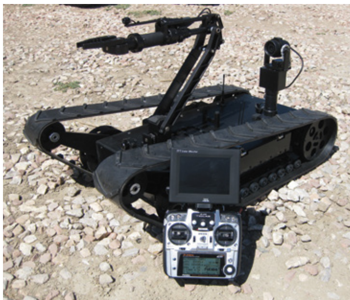
The mechanical mobility platform provides a significant degree of agility and manipulation in an economical, lightweight design. To control costs, the base unit does not incorporate feedback or processors but leverages direct operator control over a wireless link. (PHOTO COURTESY THE MACHINE LAB)
