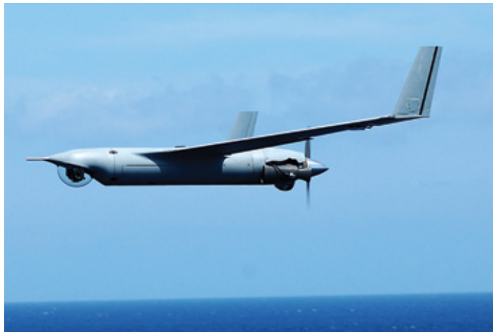
The sensor turret (left) on the ultralight UAVs weighs 700 g. (COURTESY OF INSITU INC.)
