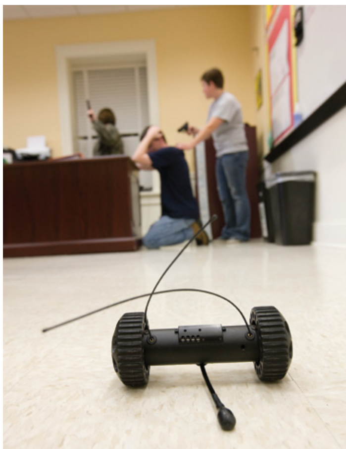
The original Recon Scout IR was designed for tactical law enforcement applications in relatively clean urban environments. (PHOTO COURTESY RECONROBOTICS INC.)
