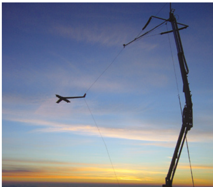
For capture, the UAV snags a wingtip on a vertical rope, for a rapid deceleration that exerts 20 Gs of applied force. (COURTESY OF INSITU INC.)
