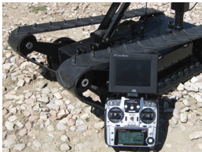
Tactical robot features a 4-axis arm on a platform that provides higher speeds and the ability to climb stairs of featuring more battery power for a factor of four increased in run time. (PHOTO COURTESY THE MACHINE LAB)
