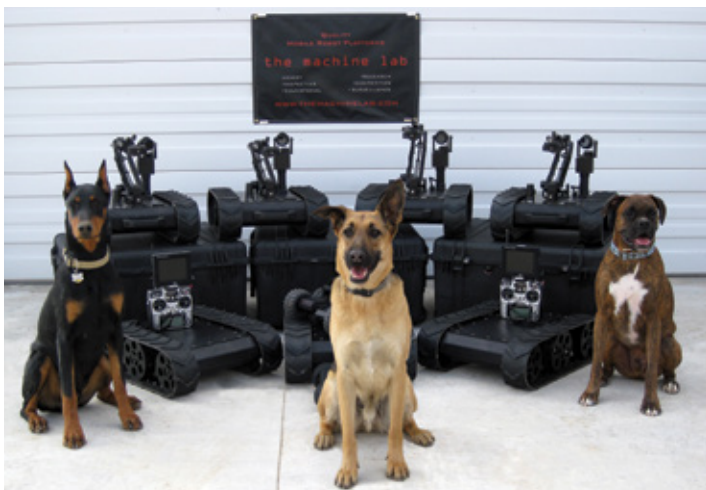
The robots range in size from 5-lb. models that can carry 4lb. payloads to significantly larger models that can carry up to 40 lb. while remaining man portable. No word on whether they are dog portable. (PHOTO COURTESY THE MACHINE LAB)
