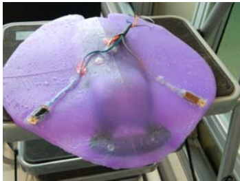
Fig. 5. Sensors are mounted on two fins of a robotic stingray
