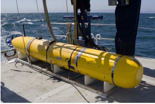
Fig. 3. MBARI mapping vehicle used to test the wall-following control.
