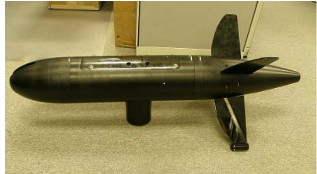
Figure 6. A Liquid Robotics tow body hosting a Teledyne Benthos PBD.
