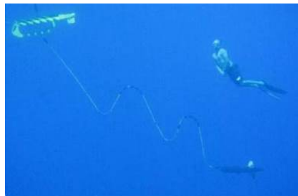
Figure 7. Undersea photograph of a Liquid Robotics Wave Glider (submarine portion) with a tow body.
