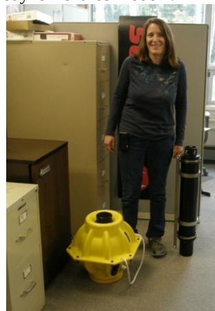
Figure 3. A 9 – 14 kHz PBD and modem housed in a 6000 m glass sphere plus a second unit in a 2000 m cylindrical housing.
