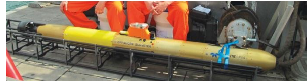
Figure 8: The Gavia AUV development system (gold modules) fitted with a production Benthos ChirpIII SBP (yellow module), on trials with UTEC Survey.
