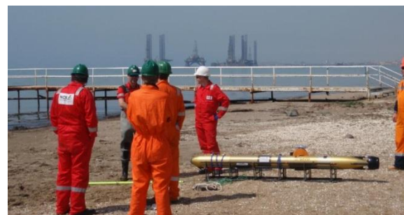
Figure 6: Gavia AUV configured for an offshore survey, with swath bathymetry, camera, side scan and INS/DVL navigation. Photograph: NCS Survey Ltd, Aberdeen UK.
