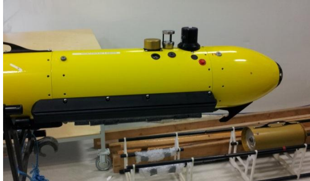
Figure 9: The Klein 3500 side scan integrated in a Gavia test module, ready for sea trials.
