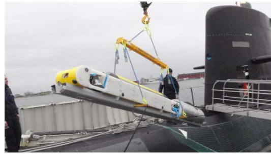
Figure 1 SUBROV being loaded in submarine.
