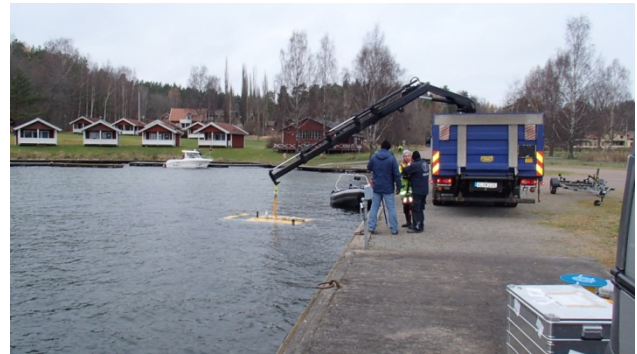
Figure 27 Sabertooth mobile test site consists of a small control van and a lorry with crane
