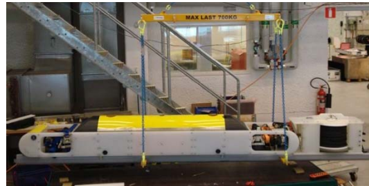
Figure 2 SUBROV on torpedo tube docking skid with winch.
