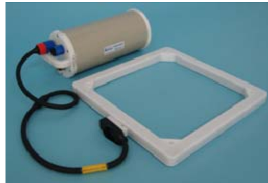
Figure 12 Example of communication antenna from WFS.
