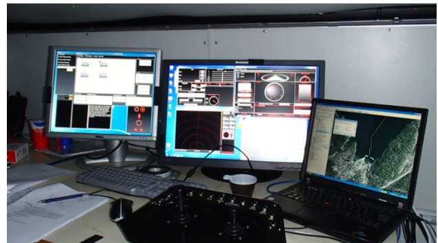
Figure 28 Sabertooth controls set up in van
