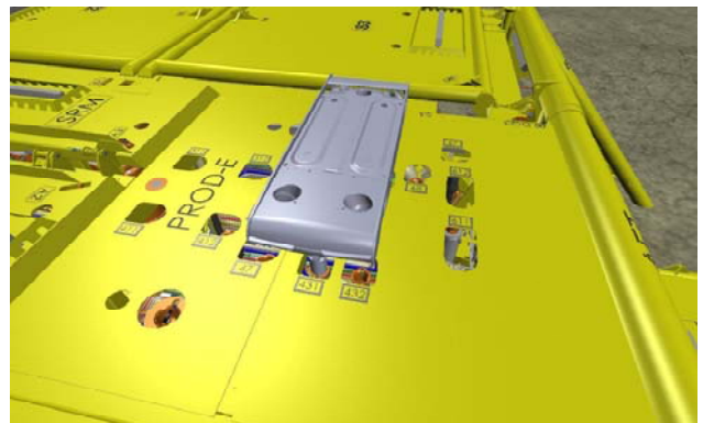
Figure 22 Sabertooth above SPS. Picture Courtesy from Aker Solutions
