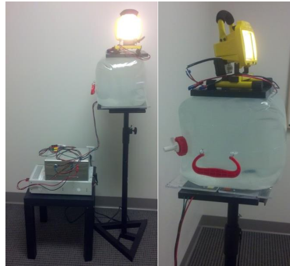
Figure 7: Image of a HR-WPT system in operation transferring power through water
