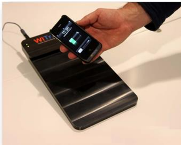
Figure 1: Photograph of a highly resonant wireless power transfer system used to wirelessly charge a battery in a smart phone (~5 W supplied wirelessly)
