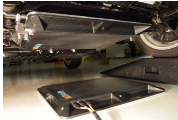
Figure 2: Photograph showing an application of HR-WPT for charging full electric and hybrid vehicles.
