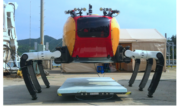
Figure 2. CR200 is standing on six legs
