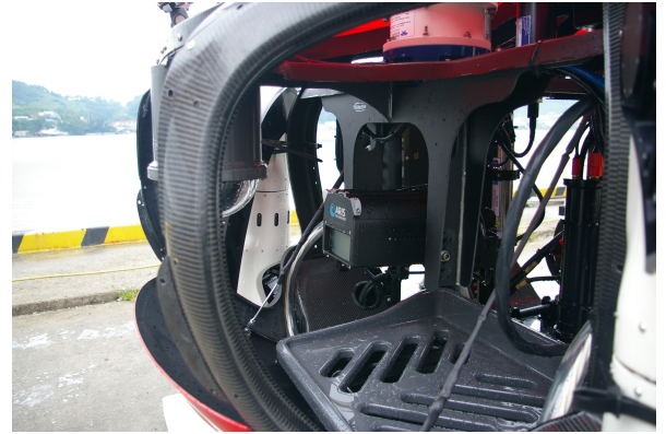
Figure 4. ARIS and X2 rotator installed on CR200
