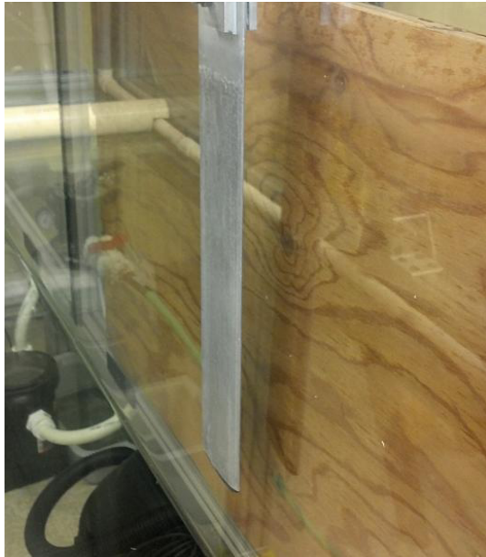
Fig. 4. Foil at closest approach to wall with height to chord ratio \frac{\bar{h}}{c} = 1.5 . With heave to chord ratio \frac{h_0}{c} = 1 , the closest approach is one half the chord length, \frac{c}{2} .
