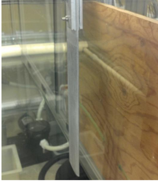
Fig. 3. Foil at closest approach to wall with height to chord ratio \frac{\bar{h}}{c} = 2 . With heave to chord ratio \frac{h_0}{c} = 1 , the closest approach is the chord length, c .
