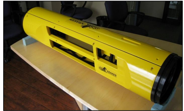
Figure 10: Kraken's REMUS600 InSAS1 Payload Module
