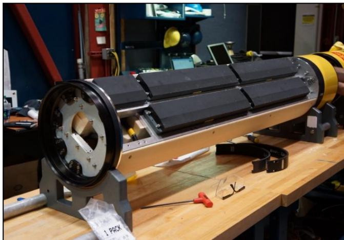
Figure 5: Single-sided InSAS2 being attached to AUV
