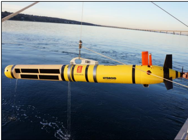
Figure 6: AquaPix InSAS2 on NUWC's REMUS600 AUV
