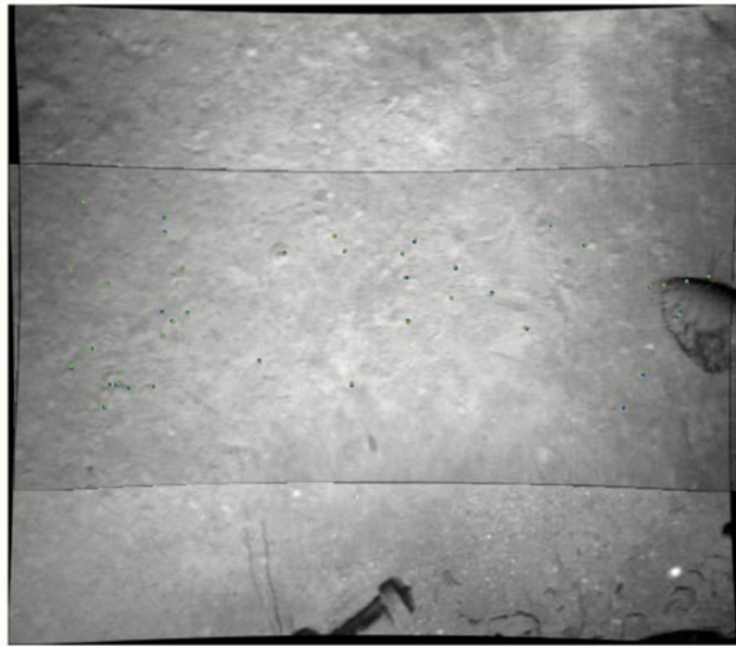
Fig. 8. Mosaic based on matching shown in Fig. 7, rendered as an average of intensities. The 41 corresponding feature points used to calculate the homographies to map onto the mosaic frame are shown in blue (top image) and green (bottom image).
