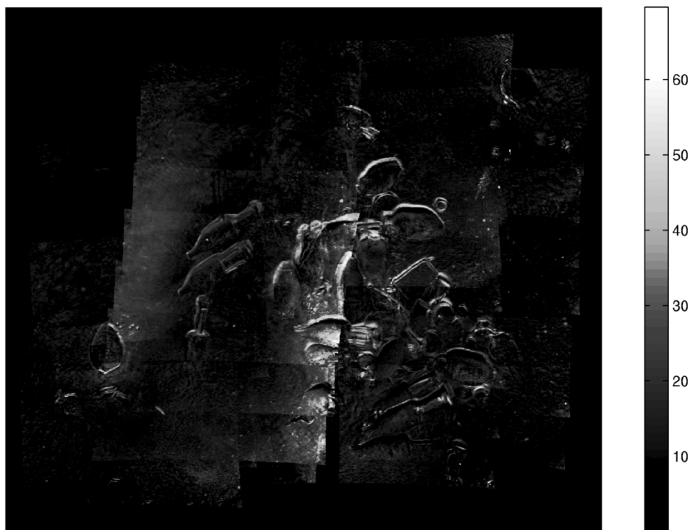
Fig. 19. Standard deviation of all radiometrically corrected source samples at each mosaic sample (Fig. 18). High variability in pixel intensities is due to misregistrations (edge-like ghosting near objects). Notice that the variability due to lighting is significantly less than in Fig. 15.
