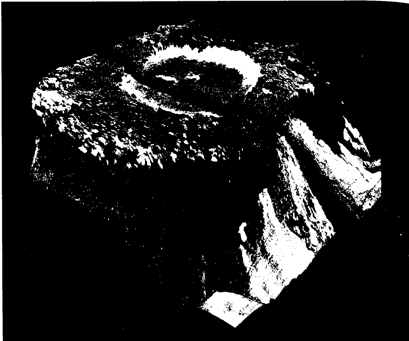
Figure 7. 3-Dimensional shaded relief presentation of combined SeaMARC I imagery and Sea Beam bathymetry. 27 Data shows a flat topped submarine volcano just off the axis of the East Pacific Rise near 13 degrees north. Figure represents a single swath of SeaMARC I imagery projected in 3-D by reference to corresponding Sea Beam Data. Seafloor depth in this image is about 2150 m, with the volcano rising 1000 m. Vertical exaggeration is 2 times. Figure courtesy of J. Farre (EPR), W. Ryan and D. Fornari (LDGO).
