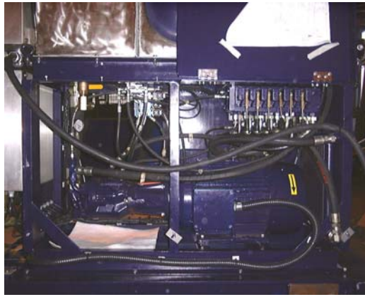
Figure 2 – Hydraulic power unit for Thales AUV LARS
