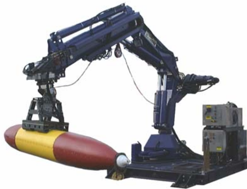
Figure 1 – AUV LARS delivered to Thales in 2001
