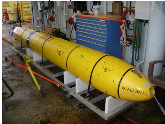
Figure 1 MBARI Mapping AUV, 17.5' Length, 21 in Diameter
