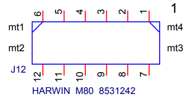
12 Positions Jack Connector 0.079" (2.00mm) Through Hole Vertical Gold With Staples
