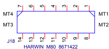
14 Positions Jack Connector 0.079" (2.00mm) Through Hole Vertical Gold With Staples
