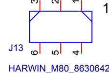
6 Positions Jack Connector 0.079" (2.00mm) Through Hole Vertical Gold
