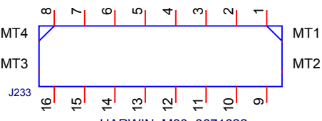
16 Positions Jack Connector 0.079" (2.00mm) Through Hole Vertical Gold With Staples
