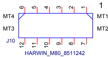
12 Positions Jack Connector 0.079" (2.00mm) Through Hole, Right Angle Gold
