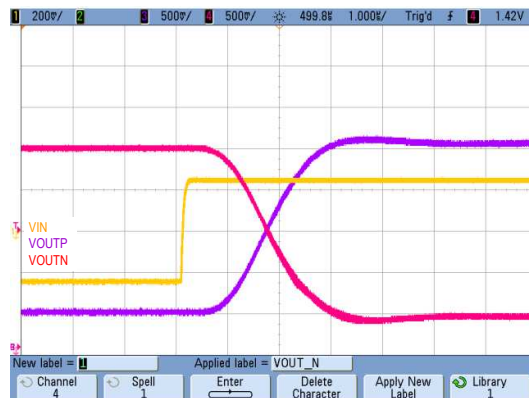
Figure 50. Step Response of the AMC1301-Q1 Device
