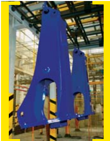
The four stage marine paint finish 1) All steel components are grit blasted to standard SA 2.5 2) KTL process – min. 40 µm 3) Intermediate layer – min. 110 µm 4) Finish coat – min. 60 µm Total dry film thickness min. 210 µm
