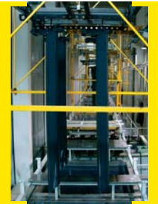
In the individual immersion tanks (13 in number) the crane parts are degreased, washed, activated, coated with zinc phosphate, washed again, de-activated and after rinsing with ultra-clean water they then undergo the electrostatic KTL coating process
