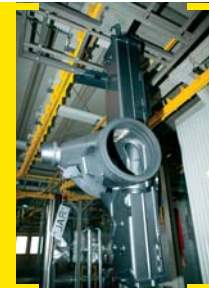
Metal shot-blasted baseframe prior to the immersion operation
