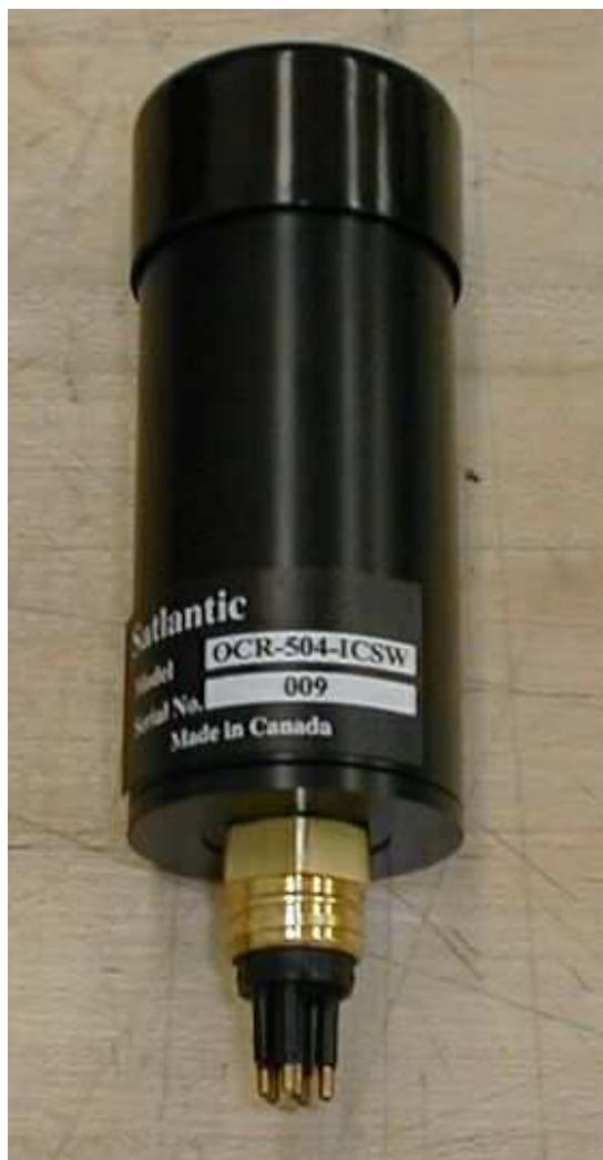
Figure 1: OCR-504 (in water) - Irradiance Configuration
