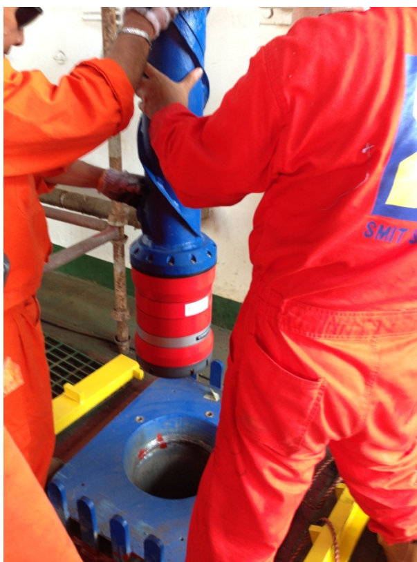
Figure 10–1 – Transceiver on Pole
