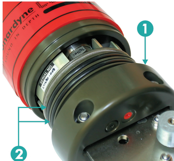
Figure 7-39 – Lubricate Sensor End-Cap O-Ring Seals
