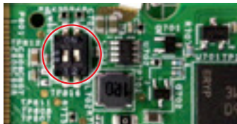
Figure 2: SW602 setting for Serial Download Mode
