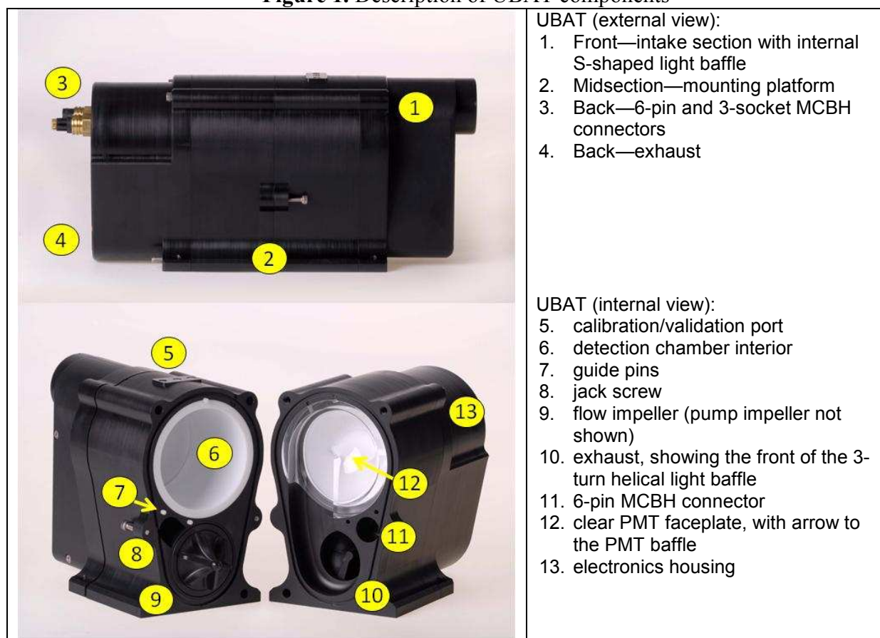
Figure 1. Description of UBAT components
