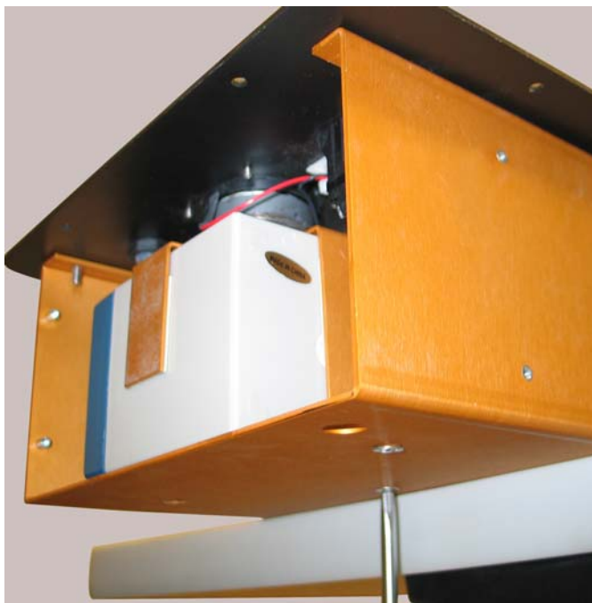
Figure 6-5 Removing the Battery Bracket Screws
