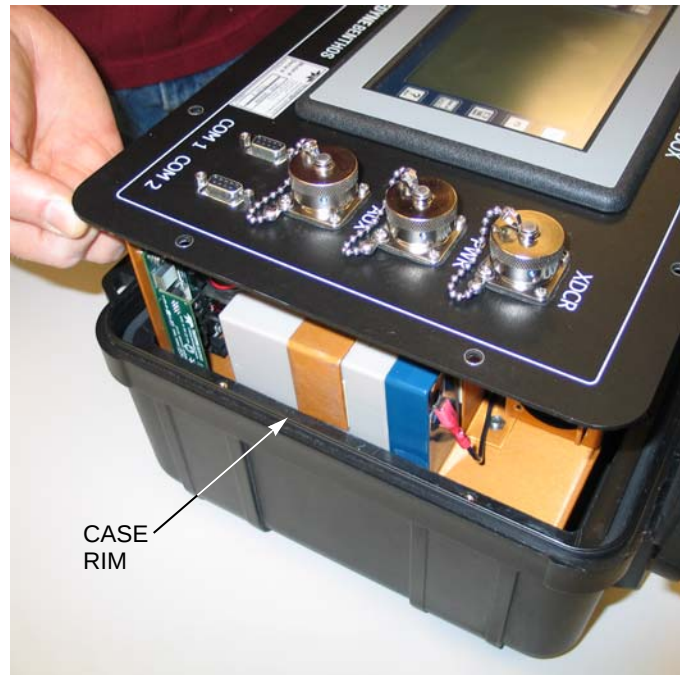
Figure 6-8 Lowering the Electronics Chassis into the Case
