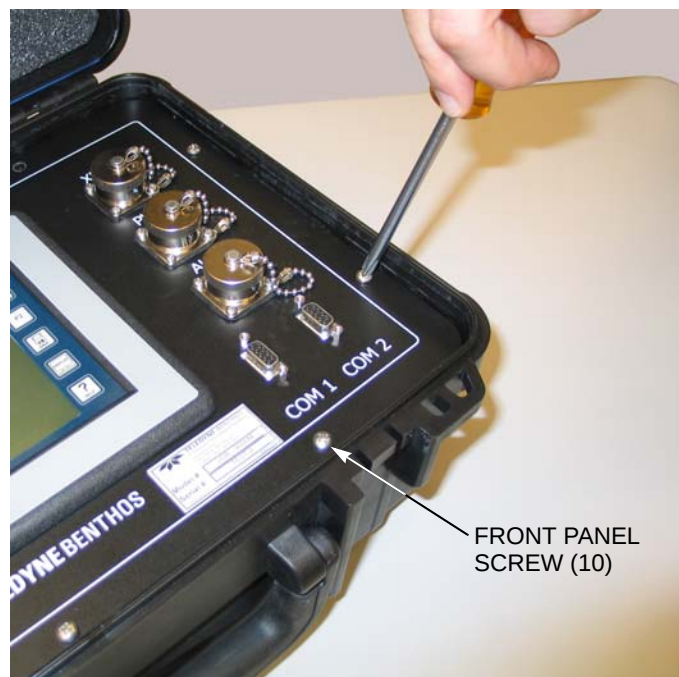
Figure 6-1 Removing the Front Panel Screws
