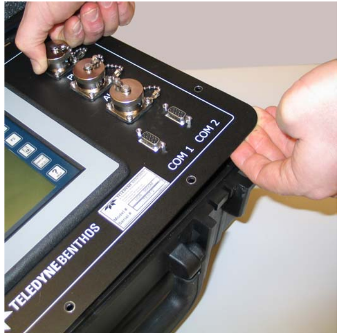
Figure 6-2 Lifting the Edge of the Front Panel
