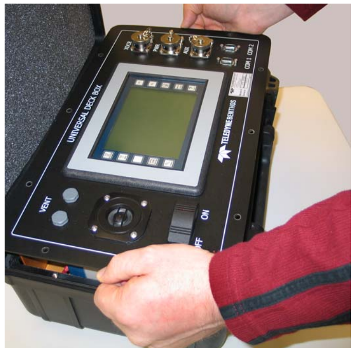
Figure 6-3 Lifting the Front Panel and Electronics Chassis Out of the Case
