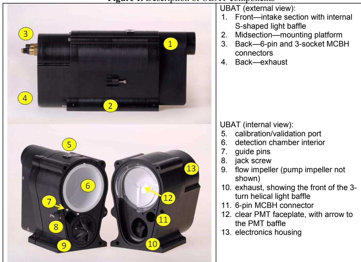
Figure 1. Description of UBAT components
