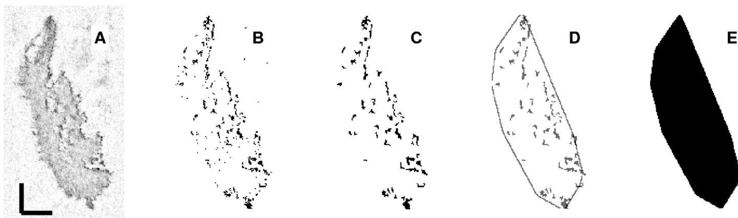
Fig. 5. Image-processing sequence performed on individual object within an ROI. An in-focus object (A) undergoes segmentation by edge detection (B). The strong edges of the object are highlighted by multiply connected pixels. Morphological closure and de-noising are performed (C) before a convex hull is fitted (D) and flood filled (E). The scale bar in A is 250 \mu\text{m} in length.
