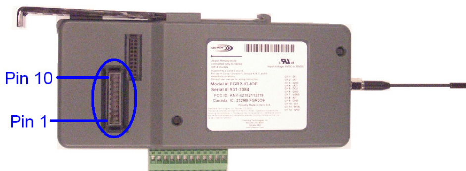
Figure 3 – FGR2-IO-IOE radio showing data connector pin numbering.
