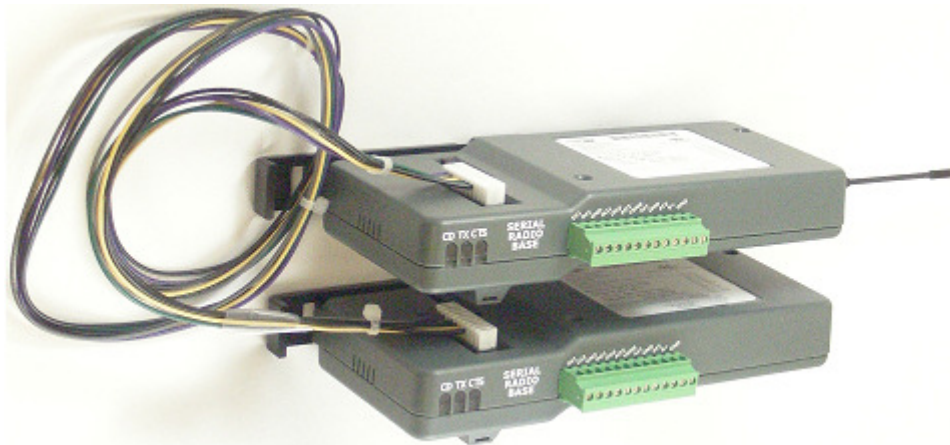
Figure 1 – Two FGR2-IO-IOE radios connected with AWR3610SP.
