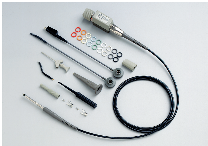
Figure 40. A typical passive probe with accessories.
