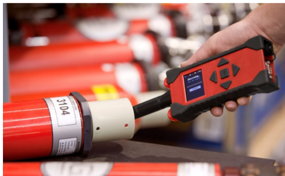
Figure 5-2 Positioning the iWAND Against the Instrument Transducer
