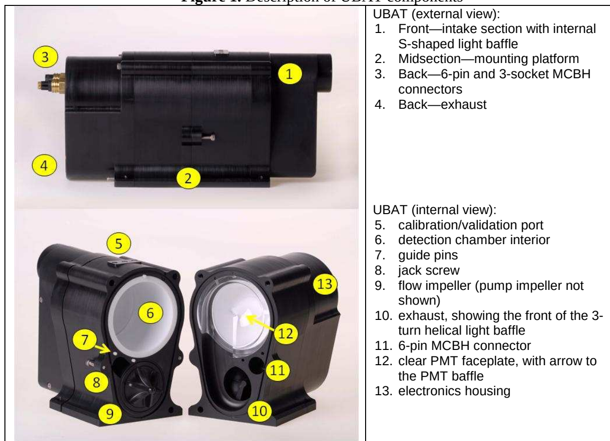
Figure 1. Description of UBAT components
