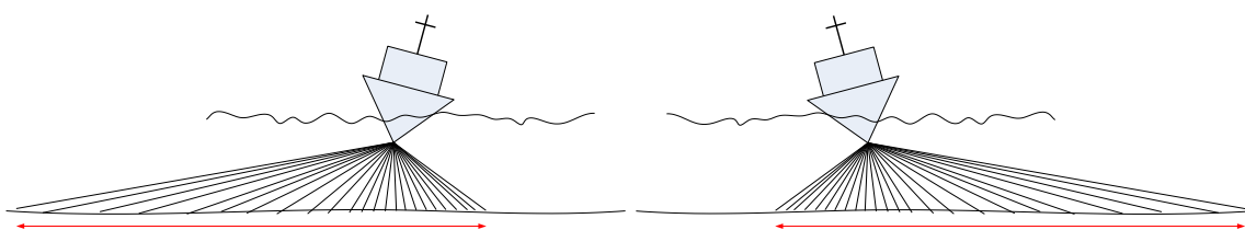
Figure 38: Laterally Displaced Swaths under Roll Conditions
