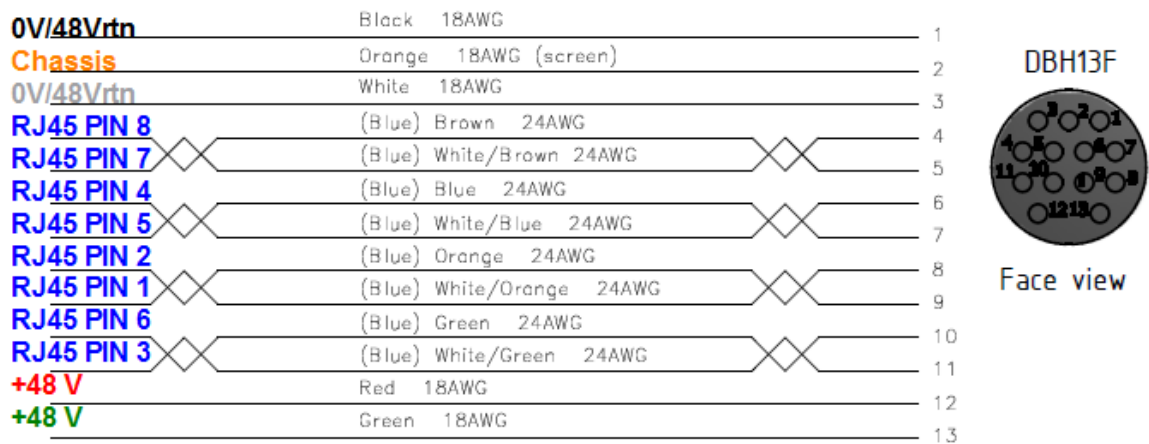
Figure 61: Bulkhead Cable Connections
