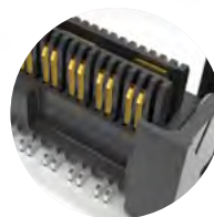
Differential Pairs Reduce Noise
