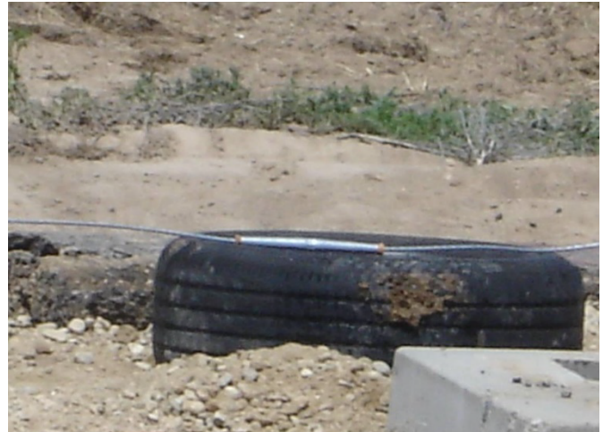
Fig. 14. A downed conductor on a tire that did not produce any arcing fault.
