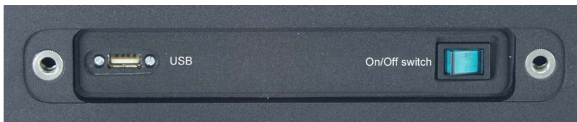
Figure 28 Connector and switch on the operator station's front
