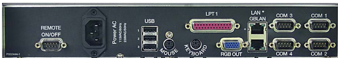
Figure 27 Connectors on the operator station's panel
