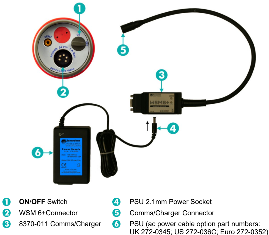
Figure 7-2 WSM 6+ Battery Charging Connections
