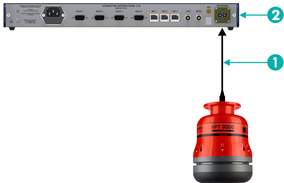
Figure 3-5 HPT to ESH Connection
